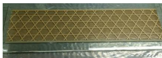
Fig. 2 Male mold placed on a layer of Teflon surrounded by four glass walls
