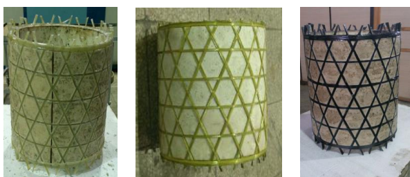
Fig. 6 Structures inside silicone mold (a) carbon-epoxy, (b) aramid-epoxy and (c) glass-epoxy
