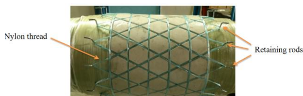
Fig. 3 Twist with nylon yarn to test the twist code
