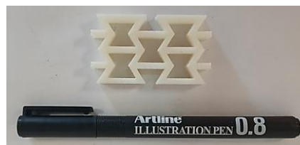
Fig. 2 As printed auxetic structure used for experiment.
