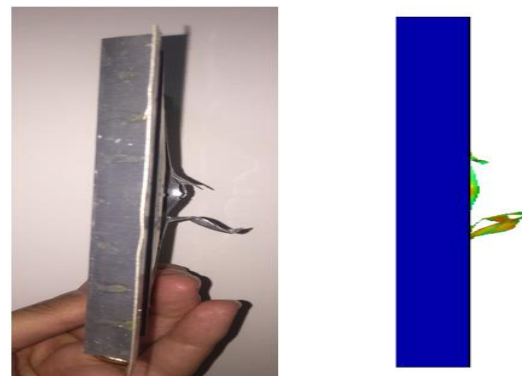
Fig. 26 Core fracture in SGE-3W3 specimen
