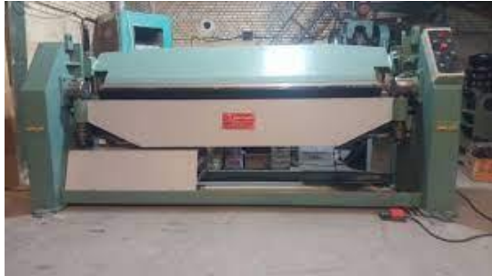
Fig. 1 Bending machine to shape the aluminum core
