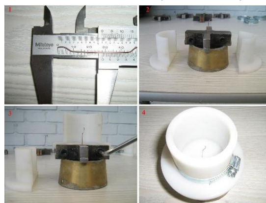
Fig. 7. Fiber installation in pull-out specimen mold
