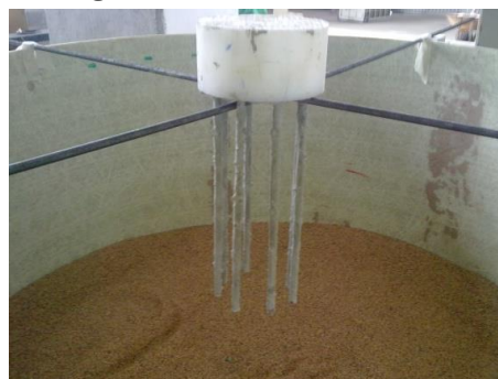
Figure (6): Solidification of cap and micro piles in the third group
