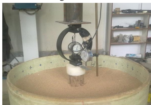
Figure (3): Sand reservoir, load ring and foundation; ready for test
