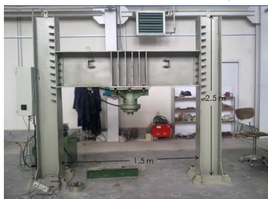
Figure (2): Reaction frame employed in the research
