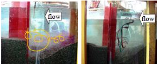
Figure 9. Flow pattern between 2 nd and the 3 rd spur dike after scouring development
