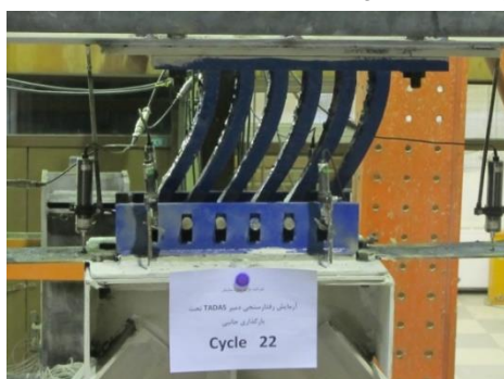
Figure 12: Damper deformation in the laboratory
