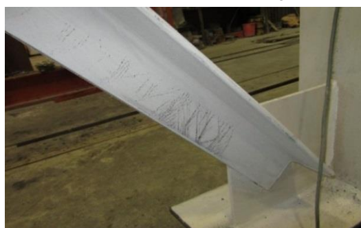
Figure 16: The brace buckling in the laboratory
