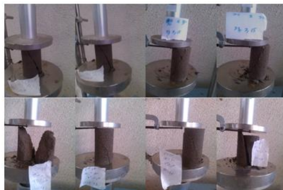
Figure 3. Failure types of stabilized specimens
