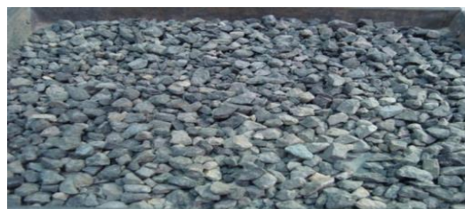
Fig. 4. Gravel used in stone column
