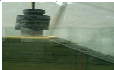
Fig. 12. Gradual loading on slope crest
