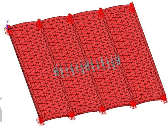
Fig. 11. The modelled jack arch roof for calibration
