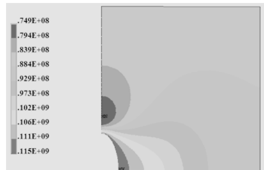
Fig. 13. von Mises stress distribution over the optimized hole using evolutionary structural optimization and nonlinear analysis
