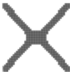
Fig. 7. Optimum shape using linear analysis
