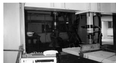
Fig. 6. Test setup slab wiremesh slab under impact load
