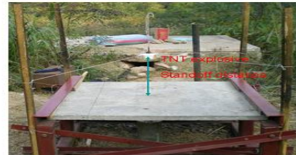
Fig. 5. Test setup slab under blast load
