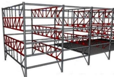
Fig. 1. Staggered truss system
