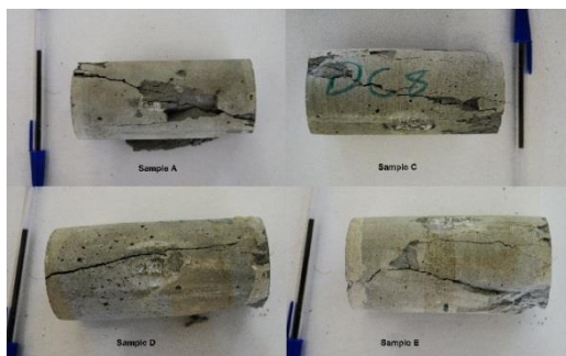
Fig. 9. Failure pattern of dry specimens with different porosity
