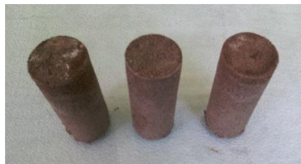
Fig. 5. Prepared samples for unconfined pressure test
