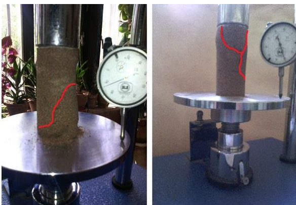
Fig. 7. Fracture of S. urea sample (right) and fracture of s. urea+B. subtilis sample (left)
