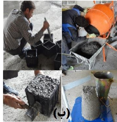
Fig. 3. Evacuation, Slump test and Molding of fresh concrete
