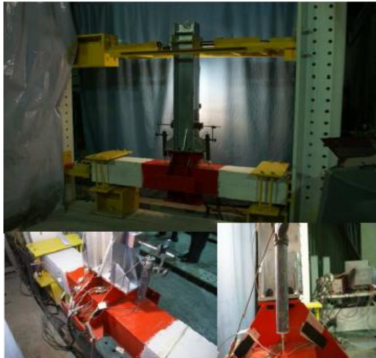
Fig. 2. Constructed composite joint
