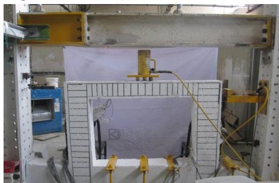
Fig. 3. loading of reference concrete frame
