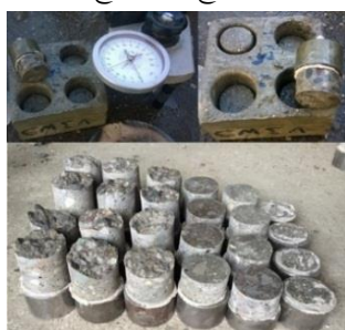
Fig. 2. Failure mode of specimens in pull-off test after freezing and thawing cycles
