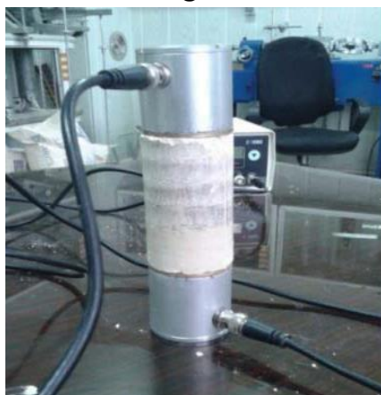
Fig. 1. Pulse generator unit and transducers for P-wave velocity measurement
