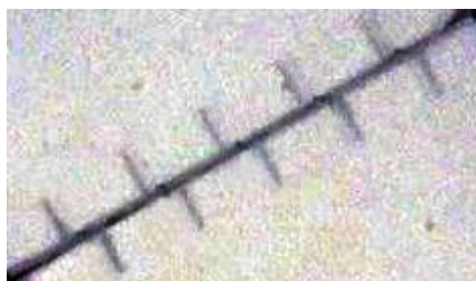
Fig. 12. Magnified image of the slip occurred between two faces of the closed flaw
