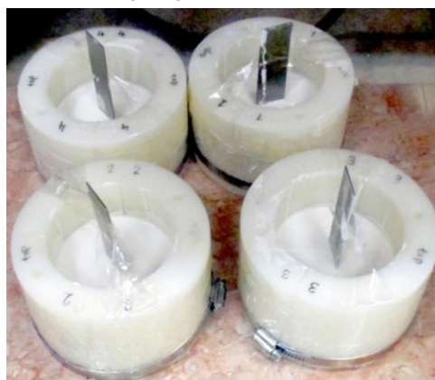
Fig. 4. Molds used to prepare specimens containing pre-existing open flaw (Steel slims inserted in the mold)
