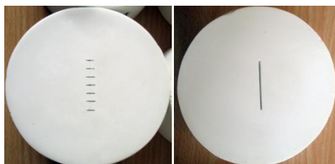
Fig. 6. Specimen containing open (right) and closed (left) flaw. Markers are used to follow slippage of closed flaw
