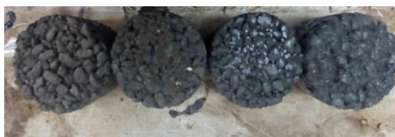
Fig. 3. Previous concrete sampels for porosity and hydrolic conductivity measurement
