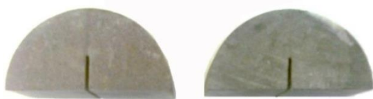
Fig. 8. SCB specimens for laboratory tests
