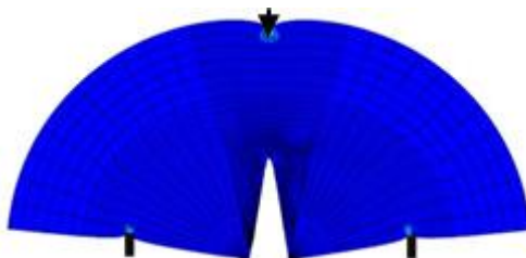
Fig. 11. Fracture path for crack after loading
