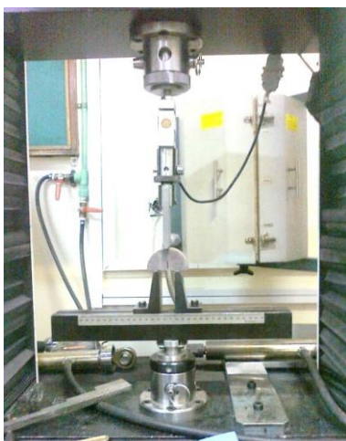
Fig. 14. Loading setup for one of the tested specimens
