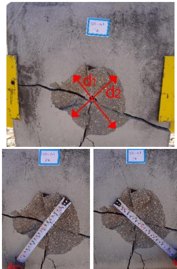
Fig. 12. Calculate the equivalent diameter of the destroyed area
