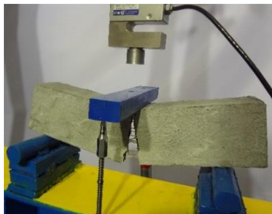
Fig. 10. Crack bending stitching by fibers
