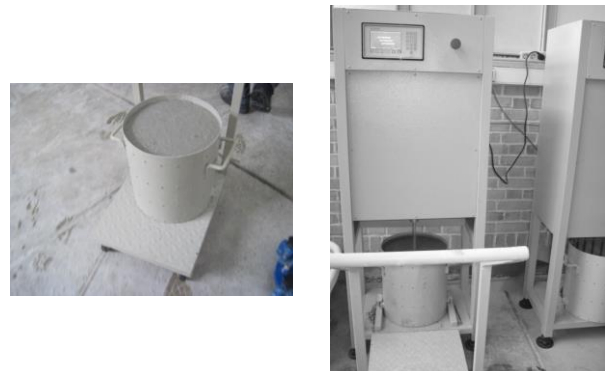
Fig. 2. Rheometer of concrete
