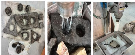
Fig. 2. Coring the asphalt concrete in the laboratory.
