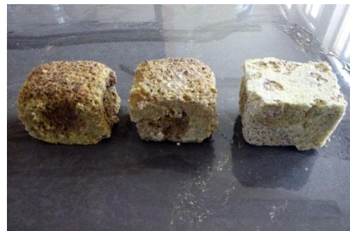
Fig. 9. Concrete samples made after exposure to acid
