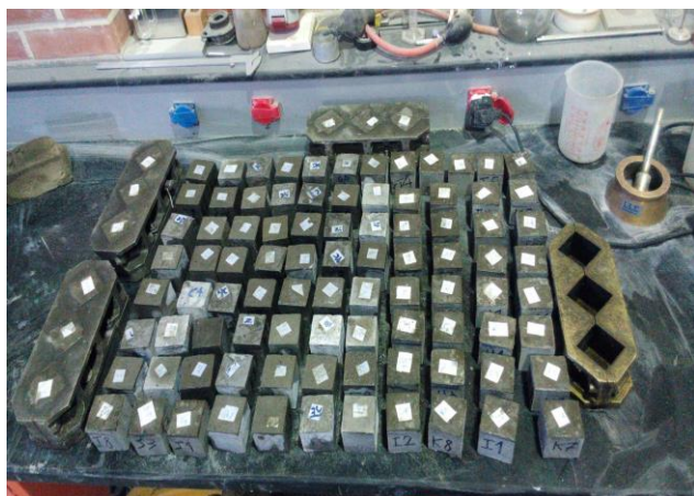
Fig. 3. Samples made of reactive powder concrete
