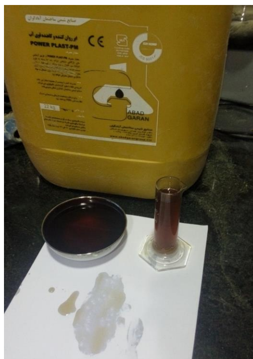
Fig. 2. The superplasticizer used in samples
