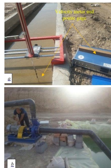
Fig. 4. a) Velocity meter and pointer gauge b) A centrifugal pump placed in field laboratory
