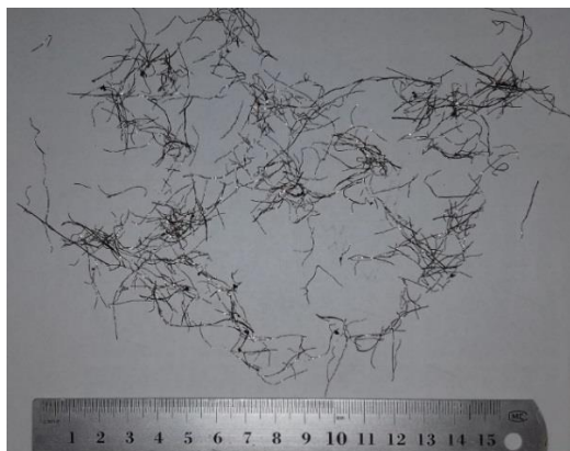
Fig. 2. Recycled still fiber from old tire
