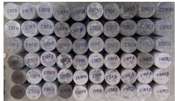
Fig. 3. Specimens for indirect tensile test and compressive strength test
