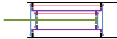
Fig. 11. Enhancing elastic deformation capacity with telescoping mechanism
