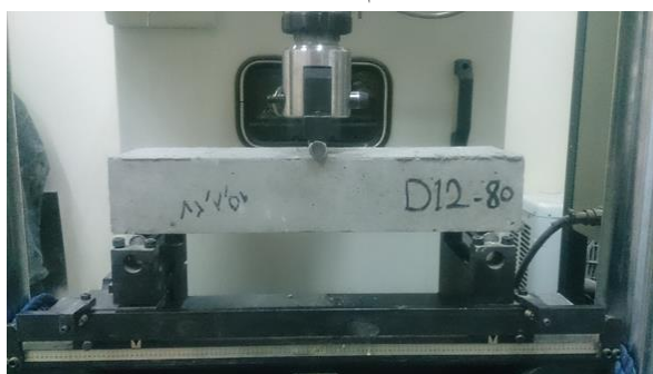
Fig. 4. Test of fatigue life of concrete samples
