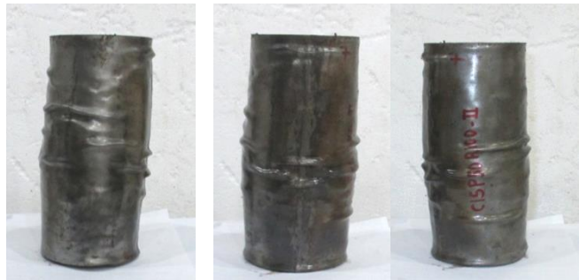
Fig. 8. Failure mode of column, 50 bar external pressure, 15 MPa concrete, D/t=100
