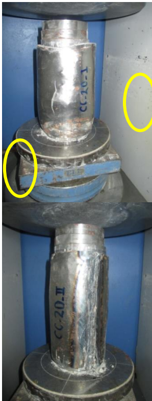
Fig. 2. Failure of specimen- Left: welding failure, right: metal failure
