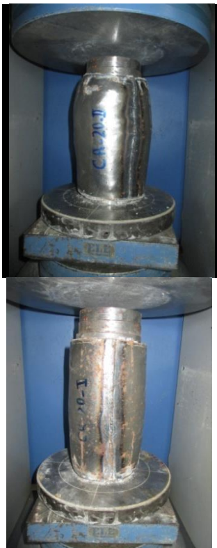
Fig. 3. Behavior of welded tube by argon welding
