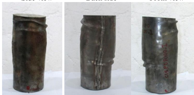
Fig. 7. Failure mode of column without external pressure, 15 MPa concrete, D/t=100
