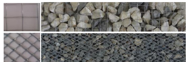
Fig.2. Grids used to make gabion spur dike
