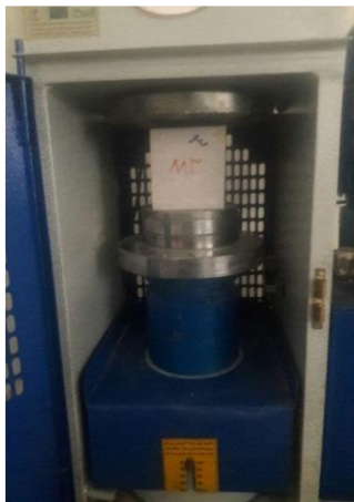
Fig. 4. Testing the compressive strength of the samples
