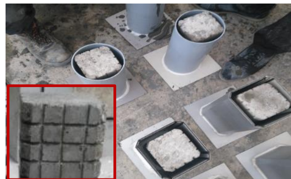
Fig. 1. Implementation of grooves and cover layer
