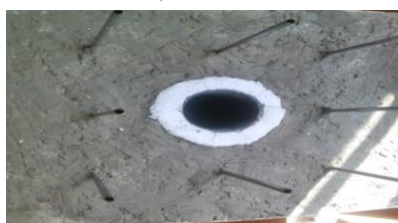
Fig. 5. Protected tube with 40mm thickness geofom
