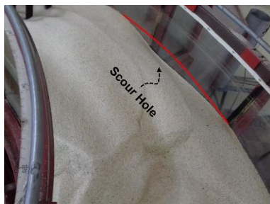
Fig. 12. An instance of the second scour hole, (D-V) I120 experiment
