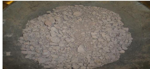
Fig. 10. Material after Oedometer test
