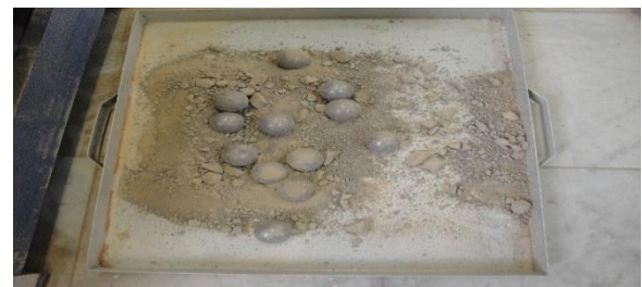
Fig. 11. Material after Los Angeles test
