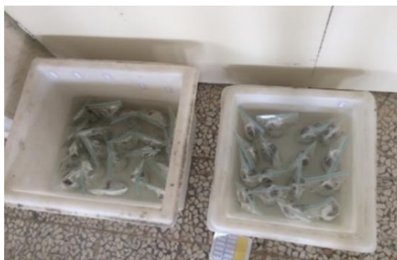
Fig. 2. Curing in a wet environment
