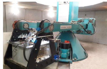
Fig. 4. Geotechnical centrifuge in University of Tehran
