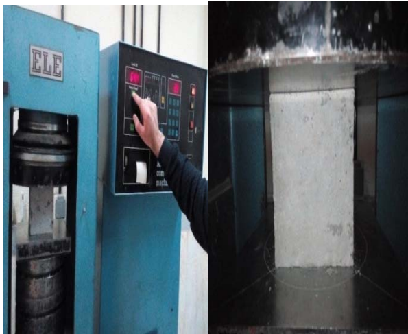
Fig. 1. Compressive strength test machine and specimen
