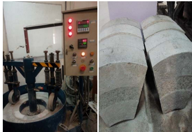
Fig. 2. Abrasion resistance test machine and specimens
