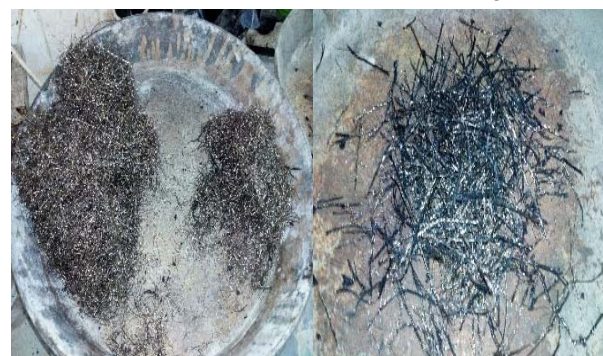
Fig. 6. Recycled steel fiber from waste tire
