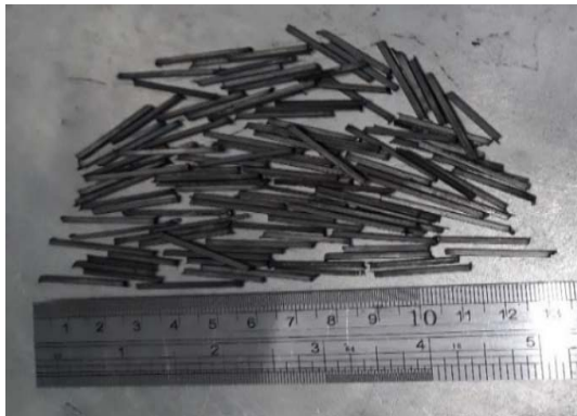
Fig. 7. Recycled steel wire from waste tire
