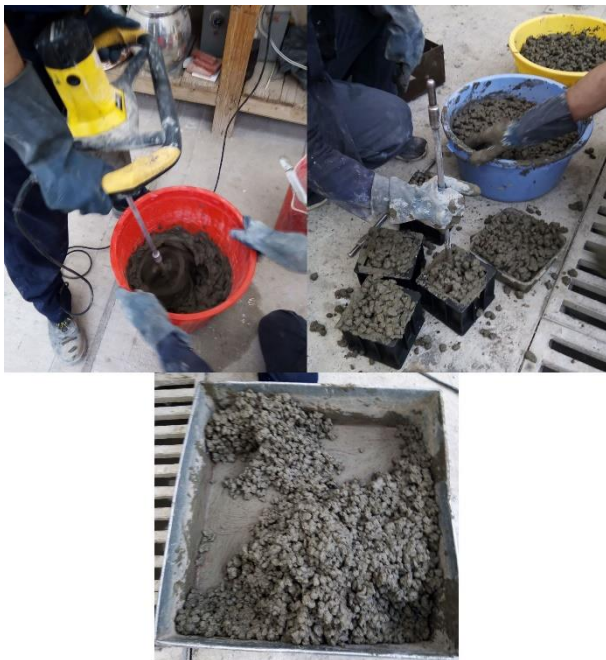
Fig. 2. Production of pervious concrete
