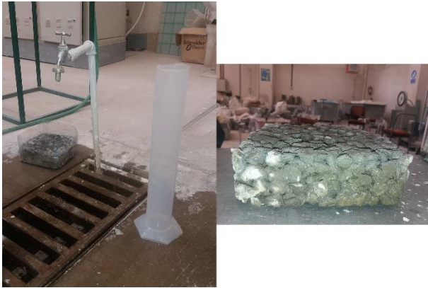
Fig. 3. Permeability test on pervious concrete
