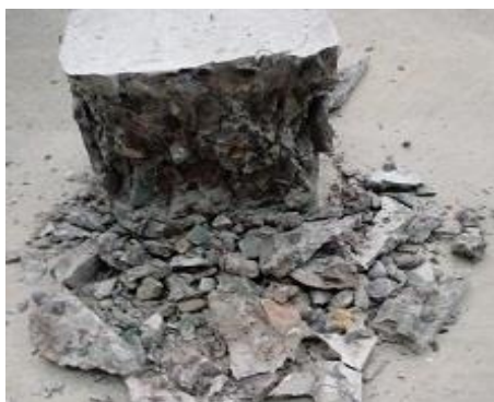
Fig. 15.b. Fracture of concrete Without fibers
