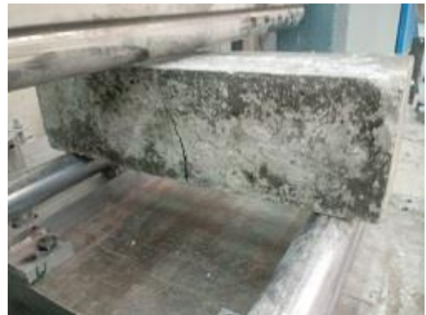
Fig. 17.a. Fracture of concrete containing fibers
