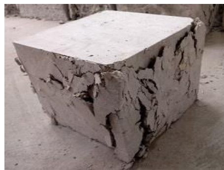
Fig. 15.a. Fracture of concrete containing fibers
