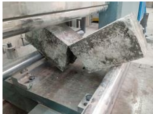
Fig. 17.a. Fracture of concrete Without fibers
