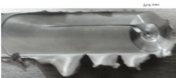
Fig. 6 Side flash on joint surface
