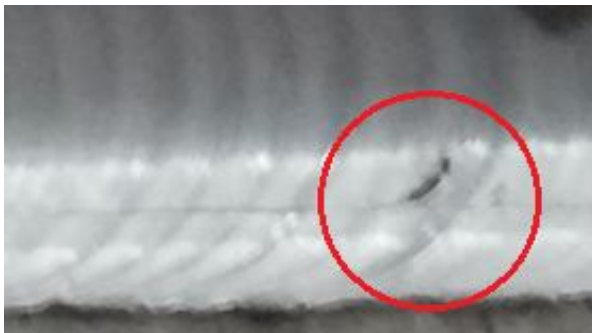
Fig. 8 Surface defect which formed in joint with 108 mm/min travelling speed
