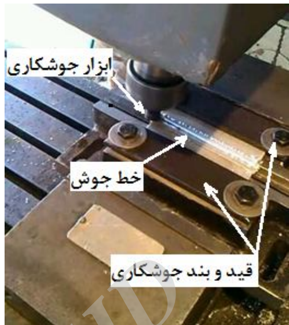
Fig. 3 FSW tool in welding progress
