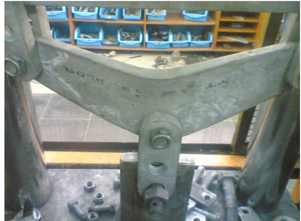
Fig. 8 Lateral buckling of yoke plate
