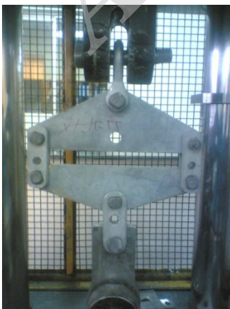
Fig. 7 Tension test set up of yoke plates
