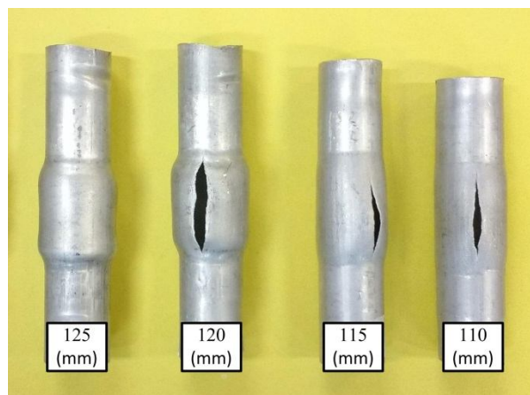
Fig. 10 Rubber-pad bulged samples with different initial lengths
