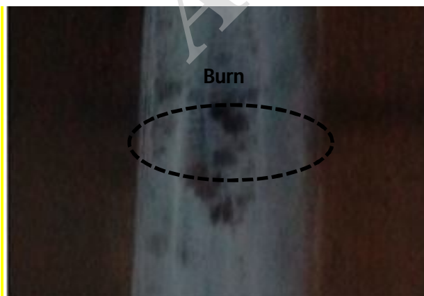
شکل 6 Creat burns on workpiece due to high rate speed
