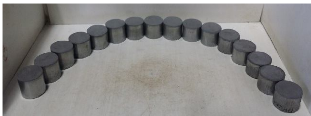
Fig. 4 Samples fabricated using dynamic compaction method
