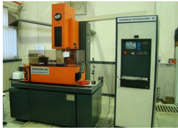
Fig. 3 Applied Charmilles EDM machine during the machining tests
