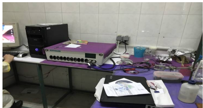
Fig. 6 An electrochemical corrosion test device used
